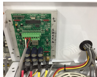
Motor speed controller DC (above the motor, under the lid of the box)
