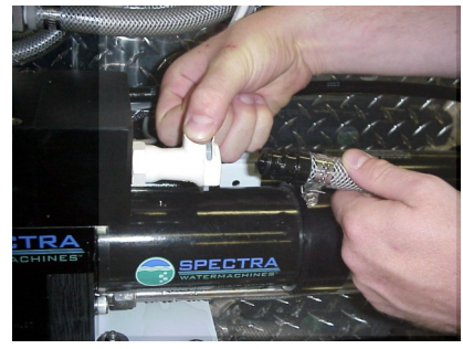
Connecting brine discharge service hose
